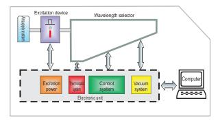
When composition elements are under excitation, spectrum with the characteristic of the element is emitted. The intensity of this spectrum has functional relation with the element content. Measure the intensity of each element spectrum to calculate the element content in material.
